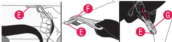
Refer to your vehicle owner's manual to locate the lower anchor bars **E** on your vehicle seat. Attach the right hook **F**, or clip **G**, to the right anchor bar **E** and the left hook, or clip, to the left anchor bar. **DOUBLE CHECK** that the lower anchor connector hook is fully engaged by pulling hard on the lower anchor connector strap.
