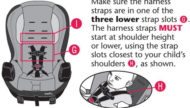
Make sure the harness straps are in one of the **three lower** strap slots **G**. The harness straps **MUST** start at shoulder height or lower, using the strap slots closest to your child's shoulders **H**, as shown.
