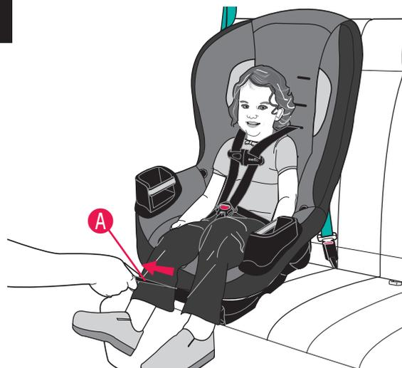
To tighten the harness straps, pull on the long harness adjuster strap **A** on the front of the seat.
