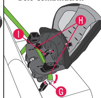
Pull the seat pad off of the front of the child restraint. Route the vehicle seat belt **G** through the rear-facing belt path **H** and continue through the opposite opening of the child restraint. **IMPORTANT:** Make sure the seat belt **G** is **in front of the crotch strap I**, and it lies flat without twisting, as shown. Fasten the vehicle seat belt, as shown, depending on your type of seat belt. Reconnect the seat pad to the front of the child restraint.
