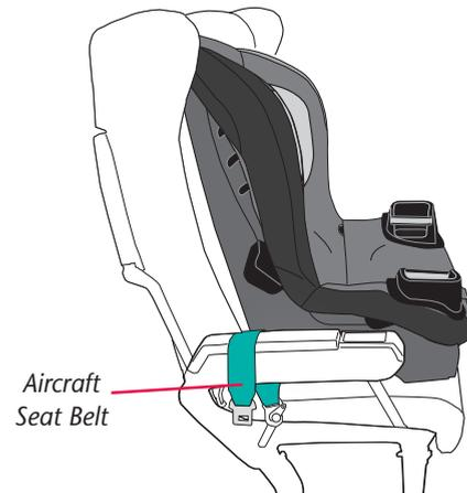
Adjust the child restraint to its **upright position** (page 38), then place it on the aircraft seat **forward-facing**, as shown above.
