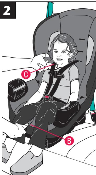
To loosen the harness straps, push the harness release button **B** on the front of the seat. At the same time, pull up on the harness strap **C** near the child's shoulders.
