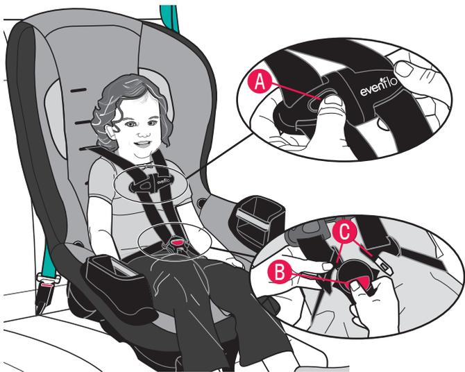
Push the release button **A** and pull the chest clip apart. Press the red buckle release **B** and remove the buckle tongues **C**.
