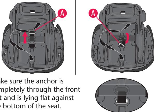
Make sure the anchor is completely through the front slot and is lying flat against the bottom of the seat.
