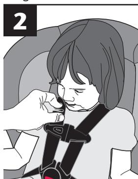
**2** The harness straps must be snug against the child. A snug strap should not allow any slack. It lies in a relatively straight line without sagging. It does not press on the child's flesh or push the child's body into an unnatural position. Check the harness straps near the shoulders for slack. You should **NOT** be able to pinch the harness (see illustration). Adjust as needed.
