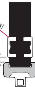
If your vehicle was built **prior to model year 1996**, and has a lap/shoulder belt that is equipped with an emergency locking retractor (ELR) AND sliding latch plate, you **MUST** use a Locking Clip. Check your vehicle owner's manual to identify which vehicle belt system is in your vehicle.
