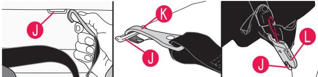
Refer to your vehicle owner's manual to locate the lower anchor bars **J** on your vehicle seat. Attach the right hook **K**, or clip **L**, to the right anchor bar **J** and the left hook, or clip, to the left anchor bar. **DOUBLE CHECK** that the lower anchor connector hook is fully engaged by pulling hard on the lower anchor connector strap.
