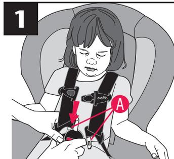
**1** Bring each harness strap over the child's shoulders. Insert the buckle tongues **A** into the buckle. Pull up on the harness strap to check that the buckle tongues are fastened.
