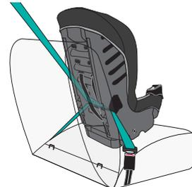
Fasten the vehicle seat belt as shown depending on your type of seat belt.
