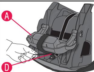
When the recline stand is in the **recline position**, wrap Velcro® strap around the recline stand **A** and insert the end of the strap through the D-ring **D**, as shown.
