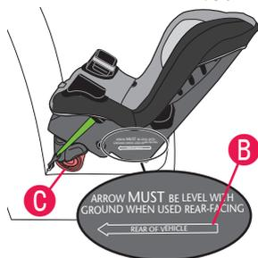
The child restraint **MUST** be in the **RECLINE** position for rear-facing use. Child **MUST** weigh 2.3 to 18 kg (5 to 40 lbs).
