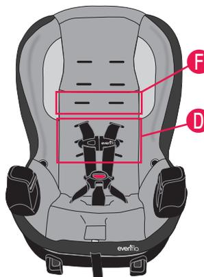
Make sure the harness straps are in one of the **three lower** strap slots **D**. The harness straps **MUST** start at shoulder height or lower, using the strap slots closest to your child's shoulders **E**, as shown.
