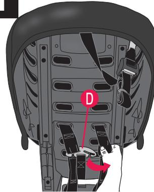
To change the harness strap position, loosen the shoulder harness as shown on page 41, step 2. Slide the harness strap off the splitter plate **D**.
