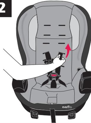
Pull harness strap through to the front of the child restraint. Thread each harness strap through the appropriate slot. Pull the harness strap to the back of the child restraint.
