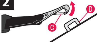
Press the tab **C** and twist, then remove the hook from the anchor **D**.
