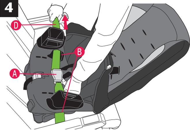
The aircraft seat belt **A** must be as tight as possible. Route the excess seat belt strap **D** back through the rear-facing belt path **B** opening, as shown above. Using your full weight, push the child restraint firmly onto the aircraft seat while pulling on the excess seat belt strap to tighten.
