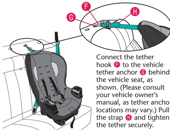
Connect the tether hook **F** to the vehicle tether anchor **G** behind the vehicle seat, as shown. (Please consult your vehicle owner's manual, as tether anchor locations may vary.) Pull the strap **H** and tighten the tether securely.
