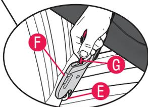
To remove the hook **C**, press the tab **D** and twist, then remove from anchor **E**.
