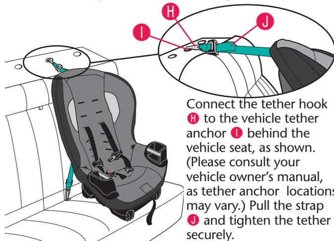
Connect the tether hook **H** to the vehicle tether anchor **I** behind the vehicle seat, as shown. (Please consult your vehicle owner's manual, as tether anchor locations may vary.) Pull the strap **J** and tighten the tether securely.
