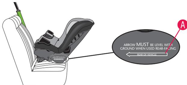
Infants **MUST** always ride facing the rear of the vehicle. Adjust the child restraint to the **recline position** (page 38). Place the child restraint in your vehicle **rear-facing**. Adjust the restraint so that the level arrow **A** is level with the ground.
