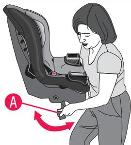
Lift the child restraint and flip the recline stand **A**, located under the child restraint seat, to either the **upright** or **recline position**.
