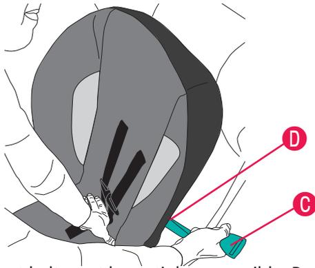
The aircraft seat belt must be as tight as possible. Route the excess aircraft seat belt strap **C** back through the forward-facing belt path **D** opening, as shown above. Using your full weight, push the child restraint firmly onto the aircraft seat while pulling on the excess seat belt strap to tighten.
