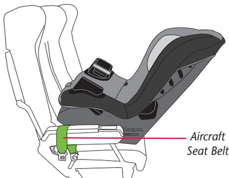
Adjust the child restraint to its **recline position** (page 38), then place it on the aircraft seat **rear-facing**, as shown above.
