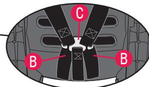
**IMPORTANT:** Make sure both harness straps are installed completely on the splitter plate, as shown.
