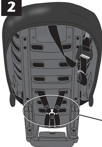
Attach the harness straps **B** to the splitter plate **C** using the **infant position** (page 37) on the harness straps. As your child grows, you can attach the harness straps **B** to the splitter plate using the pockets at the end of the straps.
