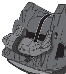
Pull until just taut and adhere Velcro to itself, as shown. (Overtightening could cause the strap to detach from the product).
