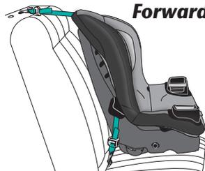
The child restraint **MUST** be in the **UPRIGHT** position for forward-facing use.
