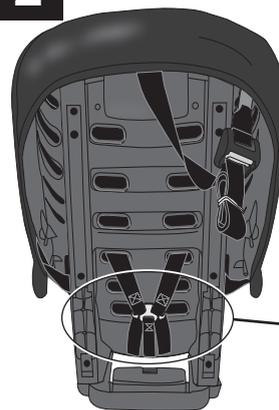
Attach the harness straps **B** to the splitter plate **C** using the **infant position** (page 37) on the harness straps. As your child grows, you can attach the harness straps **B** to the splitter plate using the pockets at the end of the straps.
