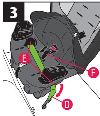
Pull the seat pad off of the front of the child restraint. Route the Lower Anchor Connector strap **D** and hook through the rear-facing belt paths **E**. **IMPORTANT:** Make sure the Lower Anchor Connector strap **D** is **in front of the crotch strap F**, and it lies flat without twisting, as shown. Reconnect the seat pad to the front of the child restraint.
