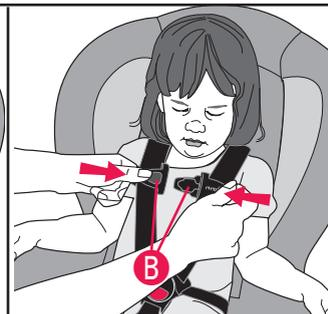
Fasten the chest clip **B** by snapping the two halves together, as shown. Slide chest clip to armpit level.
