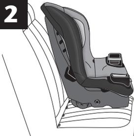
Adjust the child restraint to the **upright position** (page 38). Place the child restraint in your vehicle **forward-facing**.
