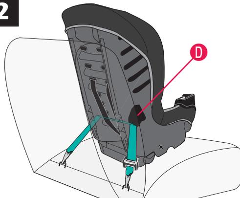
Adjust the child restraint to the **upright position** (page 38) and place it in your vehicle **forward-facing**, as shown. Route the Lower Anchor Connector Assembly through each side of the forward-facing belt path **D**.
