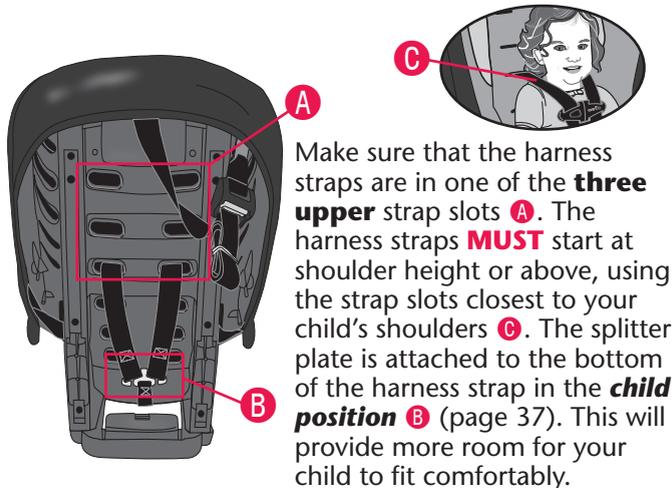
Make sure that the harness straps are in one of the **three upper strap slots** **A**. The harness straps **MUST** start at shoulder height or above, using the strap slots closest to your child's shoulders **C**. The splitter plate is attached to the bottom of the harness strap in the **child position** **B** (page 37). This will provide more room for your child to fit comfortably.
