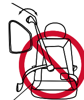
Lap-shoulder belts with top or bottom anchor points on the vehicle door.
