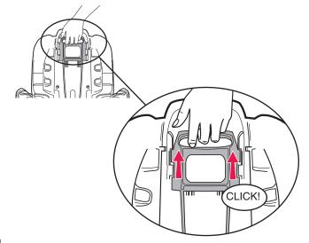
Assemble the backrest. Slide adjustment track into backrest assembly while squeezing handle. Make certain adjustment track can slide freely into different positions.
