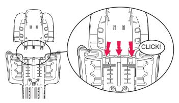
2. Install adjustment handle. Align tabs on adjustment handle with the slots on the back of the headrest. Press adjustment handle against the back of the headrest and slide upward until the tabs click into place.
