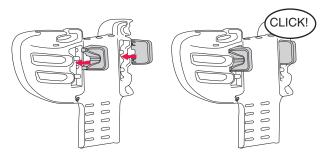
To install the Booster Inserts, line up the tabs to the slots at the rear of the backrest. Slide the Booster Inserts onto the backrest. Make certain the Booster Inserts lock into place with an audible click.
